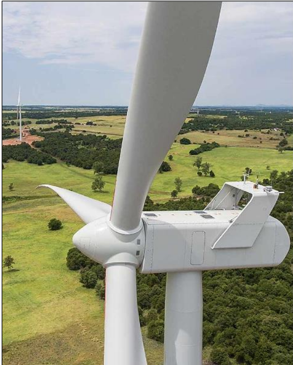
Figure 2.10: Turbine Nacelle, Hub and Blades ( https://www.enelgreenpower.com/learning-hub/renewable-energies/wind-energy/wind-turbine )
